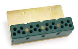
Riv-Nail Guide Blocks are available in 20- and 40-rivet capacities. Lightweight, wear-resistant UHMW polyethylene and pilot nail guides provide the most accurate placement of rivets in the belt splice.
