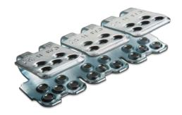
**R-5½ Rivet Fasteners** are used on belts from 9.4 to 15.1 mm thick and up to 140 kN/m. Hinge pins are found on pages 20 to 23. Riv-Nail selection can be found on pages 18 to 19.
