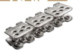
**R-5 Rivet Fasteners** are used on belts up to 11.1 mm thick and 79 kN/m. Hinge pins and Riv-Nail selections are made according to belt thickness and style. See pages 18 to 23.
