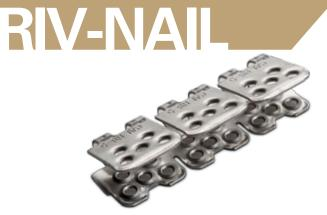
**R-5 Rivet Fasteners** are used on belts up to 11.1 mm thick and 79 kN/m. Hinge pins and Riv-Nail selections are made according to belt thickness and style. See pages 18 to 23.
