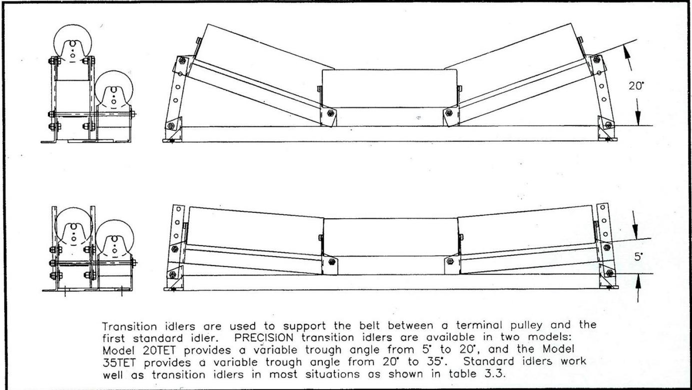
Transition idlers are used to support the belt between a terminal pulley and the first standard idler. PRECISION transition idlers are available in two models: Model 20TET provides a variable trough angle from 5° to 20°, and the Model 35TET provides a variable trough angle from 20° to 35°. Standard idlers work well as transition idlers in most situations as shown in table 3.3.
