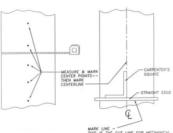
THIS IS THE CUT LINE FOR MECHANICAL FASTENER SPLICES. IT CAN ALSO BE USED FOR ESTABLISHING REFERENCE LINES FOR VULCANIZED SPLICES.
