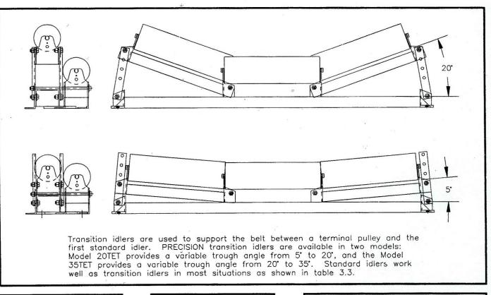
Transition Distance Terminal .1/2 Trough Pulley\_ Depth TABLE 3.1 b=Belt Width PULLEY AT 1/2 TROUGH DEPTH Idler % Rated Fabric Steel Belts Cable Angle Tension Over 90 0.9b 2.0b 0.8b 1.6b 20° 60 to 90 < than 60 0.6b 1.0b 1.6b 3.4b Over 90 35 60 to 90 1.3b 2.6b 1.0b < than 60 1.8b Over 90 2.0b 4.0b 60 to 90 1.6b 3.2b 45 < than 60 1.3b 2.3b
