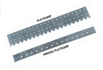
**Repair Plates** are used to prolong life of belts that have been torn, require patching of worn spots, or have "soft spots." Repair plates should be used only across the belt and never applied so they travel lengthwise over the pulley.
