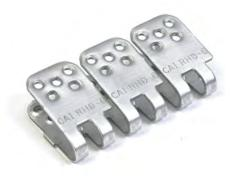
**R-6 Rivet Fasteners** are used on belts from <sup>13</sup>/<sub>32</sub>" to <sup>3</sup>/<sub>4</sub>" thick and up to 1,000 PIW. Hinge pins are found on pages 23 to 25. Riv-Nail selection can be found on pages 18 to 20.
