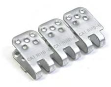
R-6 Rivet Fasteners are used on belts from  $^{13}/_{32}$ " to  $^{3}/_{4}$ " thick and up to 1,000 PIW. Hinge pins are found on pages 23 to 25. Riv-Nail selection can be found on pages 18 to 20.
