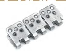
**R-5 Rivet Fasteners** are used on belts up to 7/16" thick and 450 PIW. Hinge pins and Riv-Nail selections are made according to belt thickness and style. See pages 18 to 23.
