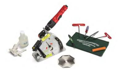
**Electric Skiver** CAI'S Electric skiving tool kit (EST-KIT) quickly skives belts for fast and easy installation of mechanical fasteners. Unit has 4 temperature settings for multiple rubber compounds. Pressure enabled contacts heat blades precisely when cutting, maximizing blade life. Clamping jaws adjust to accept blade widths from 2mm to 22mm. Unit is 110V A/C.
