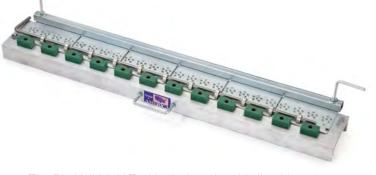
The Riv-Nail Multi-Tool is designed and built with lightweight aluminum and ultra-high molecular weight (UHMW) polyethylene locator guides mounted directly on the top of the channel. Patented anvil plates set the rivets.
