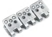
**R-5 Rivet Fasteners** are used on belts up to 7/16" thick and 450 PIW. Hinge pins and Riv-Nail selections are made according to belt thickness and style. See pages 18 to 23.
